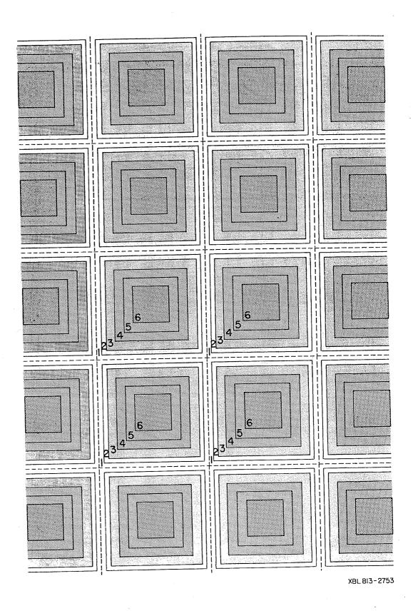
Figure 2. Basic computational mesh for a fractured porous medium.
