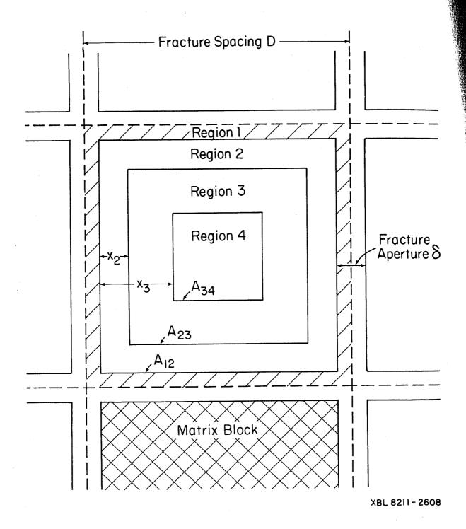
Figure 4. MINC-partitioning for an idealized fracture system.
