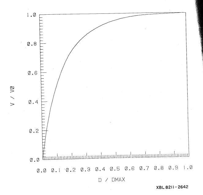
Figure 18. Proximity function for stochastic fracture distribution.
