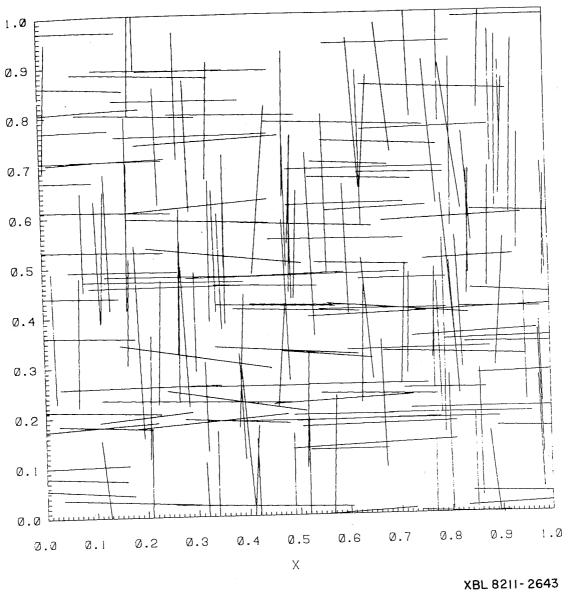
Figure 17. Two-dimensional stochastic fracture distribution.
